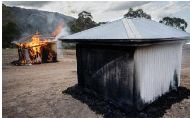
Shed with FSA Firecoat paint vs shed without in controlled real life burn situation
